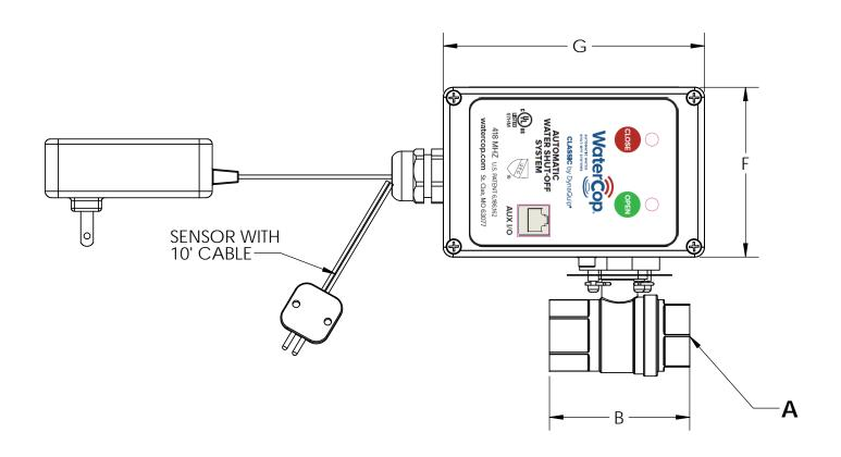
**NOTE: WCDACTHW HAS 1 SENSOR CABLE ATTACHED** WCDACTHW2 HAS 2 SENSOR CABLES ATTACHED
