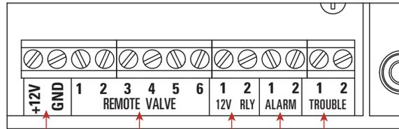
**Dry contact closure signal to security panel during alerts**
