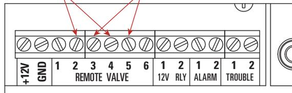
**Note:** When using WPC or WPCH to only control a remote replay (no WPACT12V attached) jumper wires must be attached as shown
