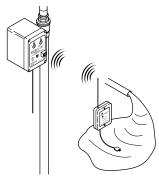
actuator instructing it to shut off the water supply to the home. The WaterCopPRO valve will remain closed until it is manually reset. The flood sensors are battery powered devices enabling them to be located anywhere a leak is likely to occur, or where water might cause damage. The WaterCopPRO actuator requires household electrical
