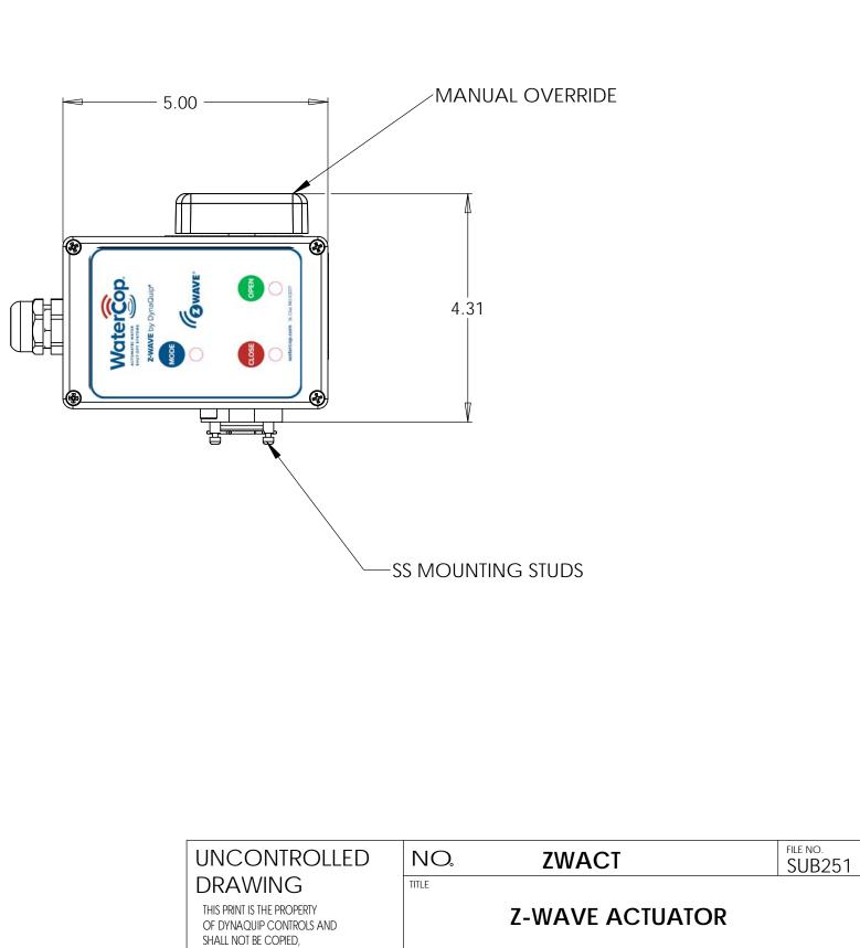
ENCLOSURE: POLYCARBONATE POWER: POWER CONVERTOR WITH 20' CORD CONTROLS: LOCAL CONTROLS WITH MANUAL OVERRIDE
