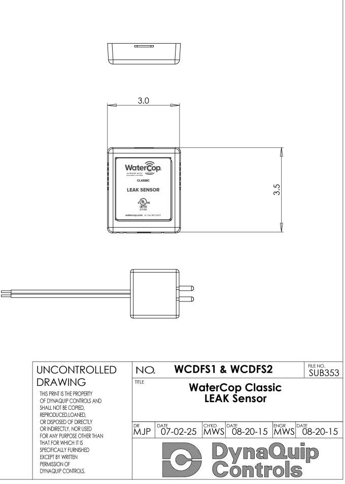
Enclosure: ABS Power Requirements: 2 AA Alkaline Batteries (Optional Power Converter) Sensor Probe: 10' Cord (Can Support 2 Probes) Mounting: Screws and Anchors Provided Frequency: 418 MHz
